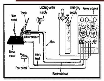
Fig. 1- Gas Tungsten Arc Welding Apparatus
