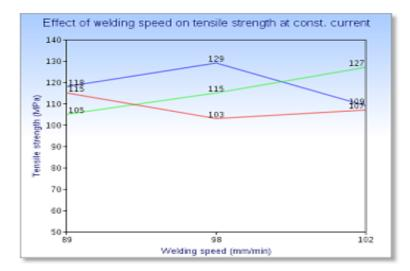
Fig. 3- Effect of welding speed on tensile strength
